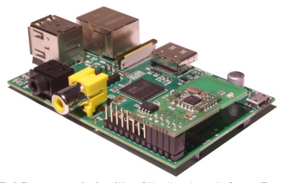
The RaZberry turns every Raspberry PI into a Z-Wave Home Automation Gateway. The bundle of hardware and precompiled Z-Wave wireless network management software waits to be completed by your own user interface running in a web browser or a mobile phone. The Z-Wave software offers an easy to understand and easy to use interface applying the well-known Javascript interface technology JSON on a built in web server. Writing your own home automation app was never easier and never more affordable.
